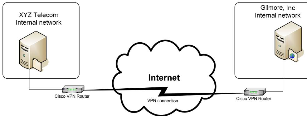
**Figure 5: Simplified VPN connection example**
