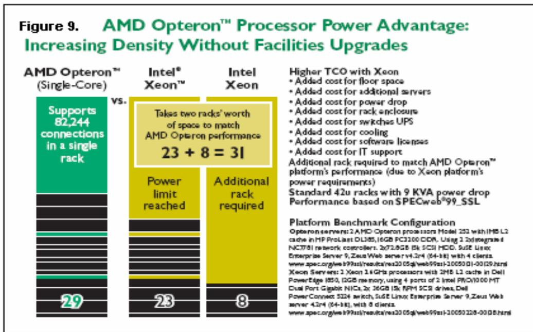
Figure 9 above, explains the advantages of low power CPUs in terms of heat density without facilities upgrades. The total power and the numbers are estimates provided by AMD, and any such comparisons need to be made in the context of a given data center with benefits measured in computing power per watt, per square foot, and in relation to the workload.
