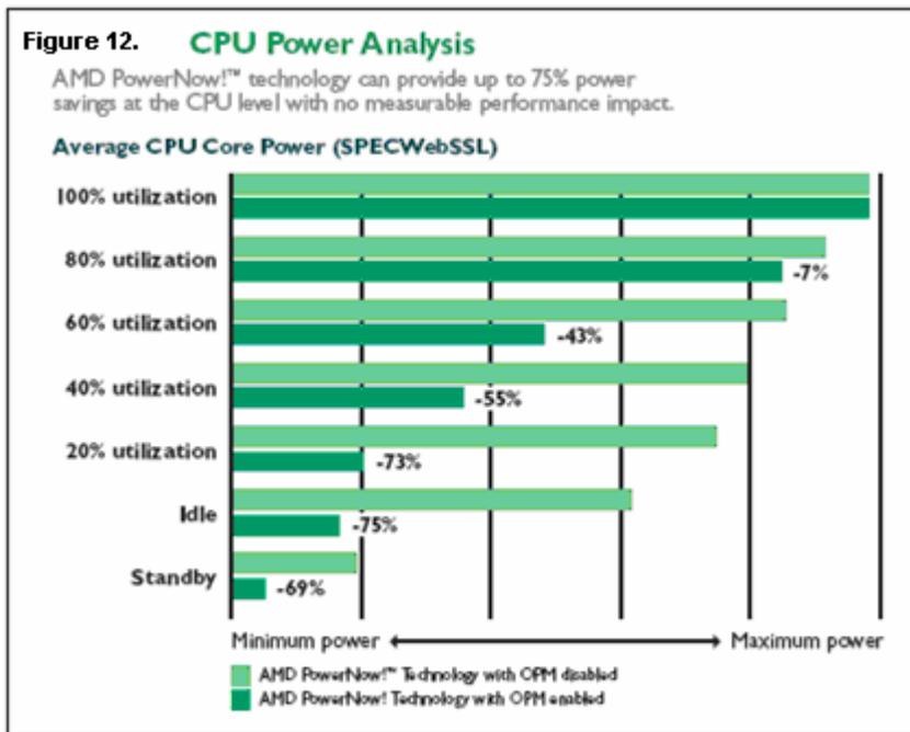
The table above shown in Figure 12, illustrates some power savings of various CPU levels with no measurable performance impact. When there is idle processor time, it can create efficiencies, but maximum power that must addressed in order to provide proper cooling.
