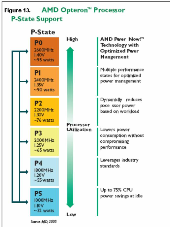
Figure 13, shows above how processor can respond to requirement changes with P-State to the lowest voltage/frequency state to reduce the thermal emissions during states of low processing requirements. Because of these lower processor states, heat do not build up unnecessarily, even in extremely discontinuous workload scenarios.
