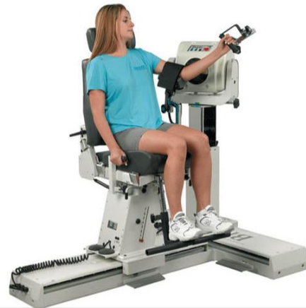
Figure 1: Cybex 770 isokinetic dynamometer cybex 770 isokinetic dynamometer for elbow - Bing images
