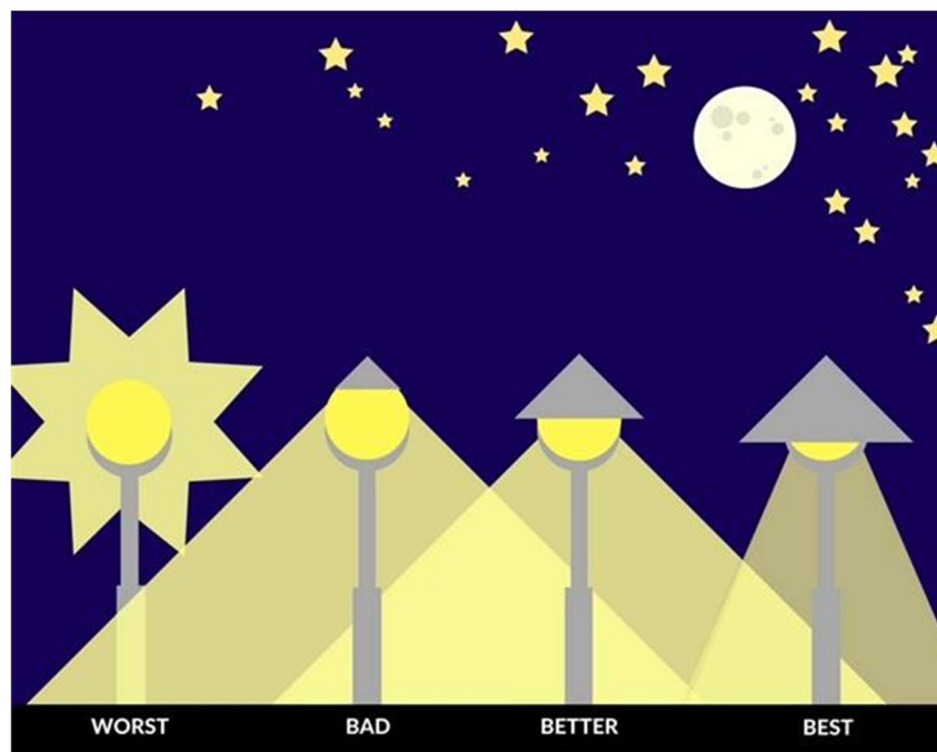
Figure 19: Properly shielded acorn luminaires reduce all four types of light pollution. (Graphic from Athens-Clarke County)
