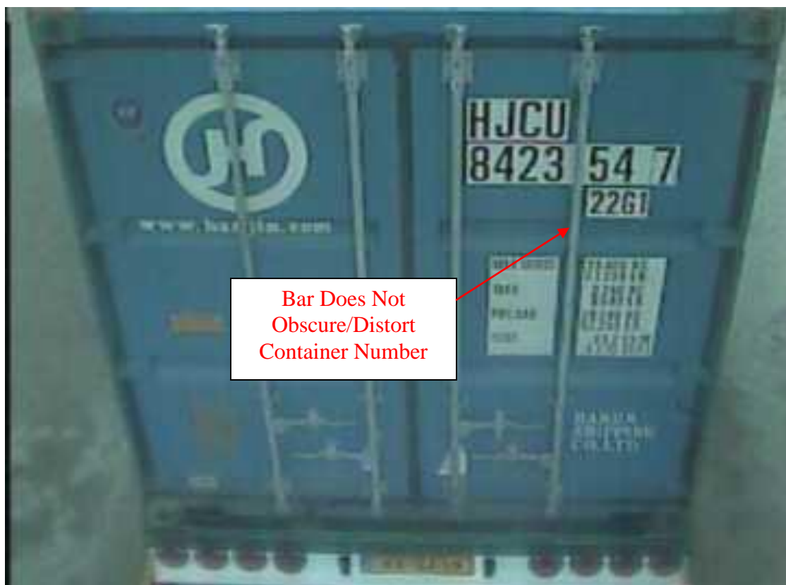
Figure 11: Non-ISO-Compliant Container When Rear Camera Not at an Angle (Katchalski, 2008)
