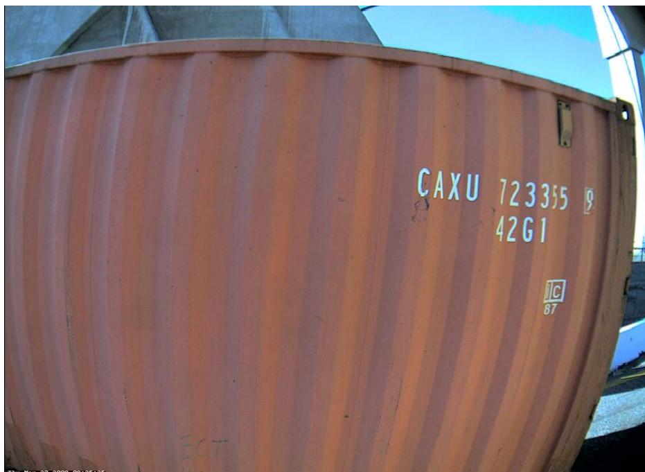
Figure 8: Example of Distorted Side Image with Current Side Camera Placement
