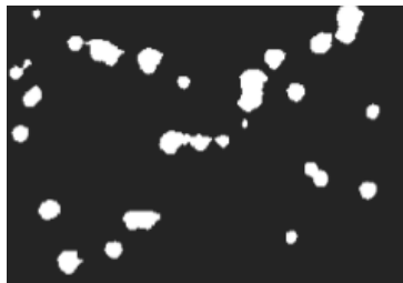
(b) Thresholded image using Otsu's.
