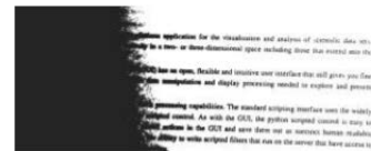
(b) Output using Otsu's method.
