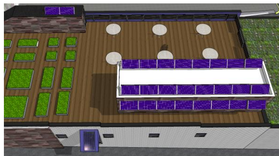
Figure 4. On-grid 8.4 kW solar energy design
