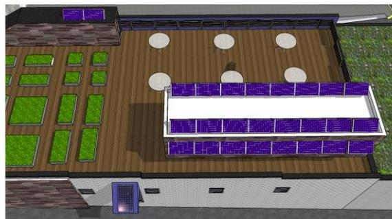
Figure 4. On-grid 8.4 kW solar energy design
