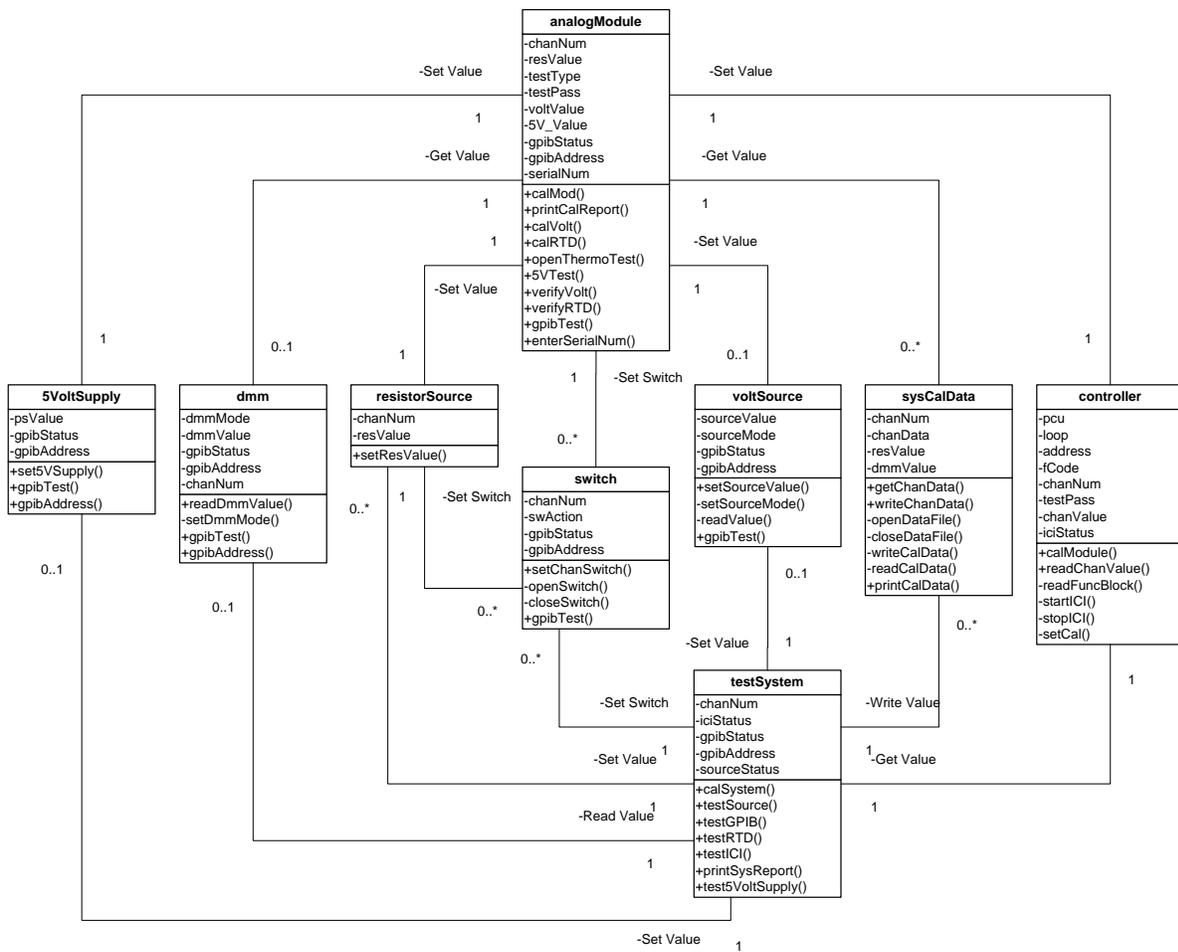
**Figure 7 - Class Diagram**
